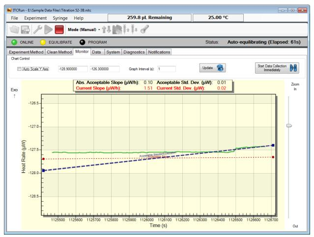
The equilibration criteria are continuously updated on the signal data chart in the Monitor tab.
