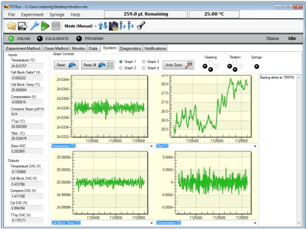
When a sample is introduced into the measurement cell, it adjusts to the instrument temperature. The graphs on the **System** tab display the status of the temperature-controlled zones of the instrument. These zones become stabilized first, followed by the heat signal which can be viewed on the **Monitor** tab.
